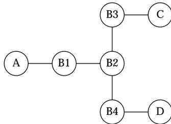
Assuming all forwarding tables are initially empty, give the forwarding tables for each of the bridges B1 to B4, after the following transmissions occur (in this order):
